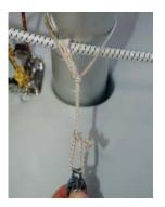
**3** Tie the air block to the mast below the boom vang tang with the piece of 3 mm Vectran (part 10).
